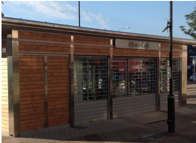
Open chain security shutters (image from the suppliers) proposal is for shutters to be colour matched to the panels.
